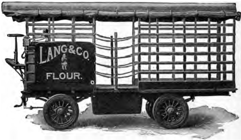
FIG. 280.—Heavy truck of the Vehicle Equipment Co. Carrying capacity, 4 tons; speed, 6 miles per hour; travel radius on one charge of battery, 25 miles.
